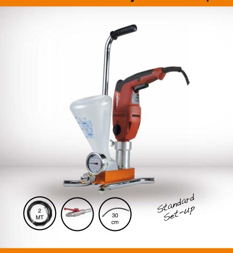
M1 is an pump light and handy designed for the injection of 1K coatings. It works by means of an electric drill. M1 is a pump for injection strong and simple construction; Lightweight and compact, easy to carry thanks to handy trolley. M1 is an equipment of great efficiency: from 0 to 250 bar in a few seconds.
